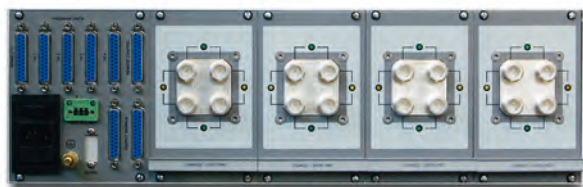
REAR VIEW GUESTS COAXIAL RELAYS AND DB25 PORTS
